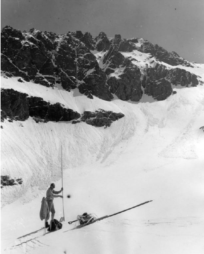
Probing snow depths on South Cascade Glacier, spring 1962. Photo by Mark Meier
